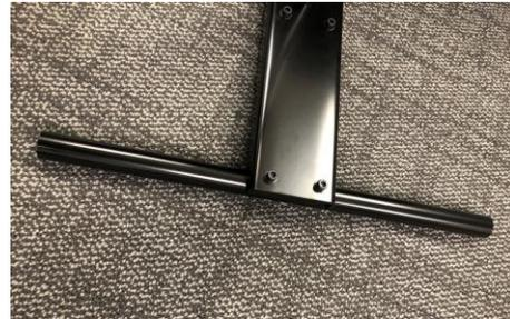
**2. Attach base plate post to base plate** by removing height adjustment lever and sliding the post up through the bottom of the base plate until its base is snug against the underside of the base plate. Place a flat washer on each of the short bolts and insert them through the top of the base plate and through the corresponding holes in the base plate post. Attach the lock nuts to each bolt and use the Hex Key and open-end wrench to tighten.
